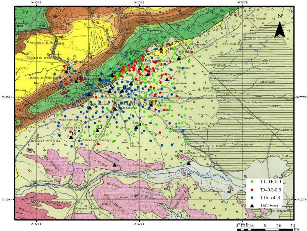
Figure 5. Peak Period of Microtremor H/V spectral ratios for all sites represented on surface geology map of Damascus city. Blue, red and green circles refer to short, medium and long peak periods respectively. Triangular refers to the location of Microtremor Array measurements.
