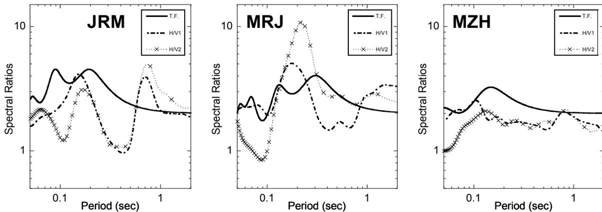
Figure 6. Microtremor H/V spectral ratios and Site Transfer Function (Vs velocity was calculated according to Y. OHTA's empirical equations, 1978) for different sites in Damascus city
