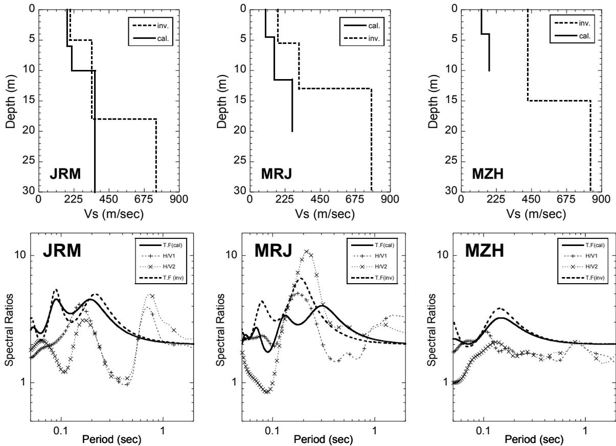
Figure 7. Upper part shows soil profiles (inverted and calculated Vs profile), while lower part shows Microtremor H/V spectral ratios with calculated site transfer function (Y. Ohta and N. Goto, 1978) and inverted one (Zaineh et al., 2010) for different sites in Damascus city
